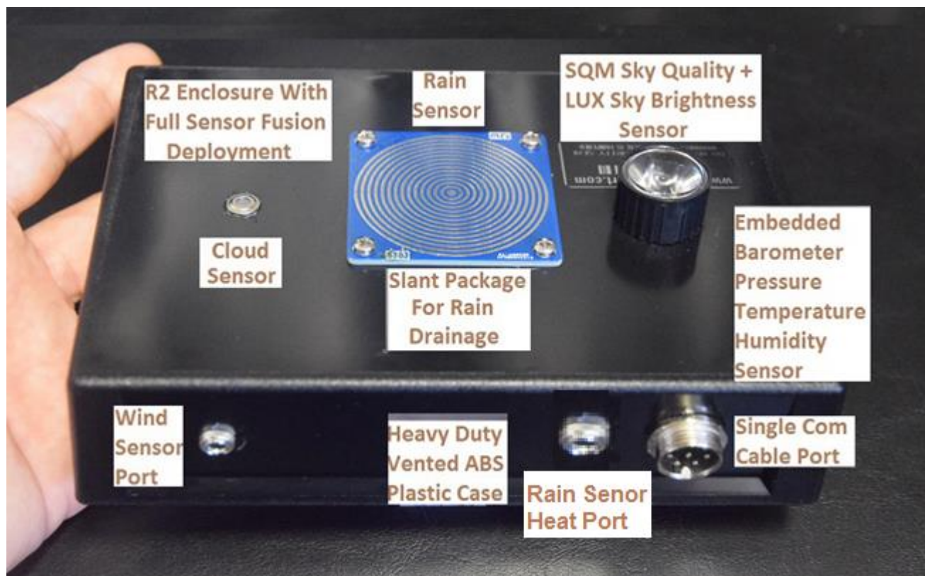
Figure 6 R2 Full Sensor Fusion Enclosure Break-Out Overview Model (2018).
