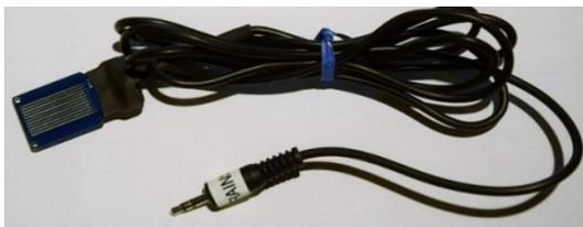
Optional accessory that Astro-Smart offers is the rain sensor ([4RAINSENSOR-RCOC-CDAP](#)). For use with RCOC-CDAP-PRO or any Astro-Smart Model with custom build option. That is correct. I can add this sensor to all variants of the CDAP-PRO model as a custom build option to new or preowned models. Goto the purchase page for this option. This sensor informs the user of rain fall when observing remotely and gives the user safety option decision making capability for the correct
