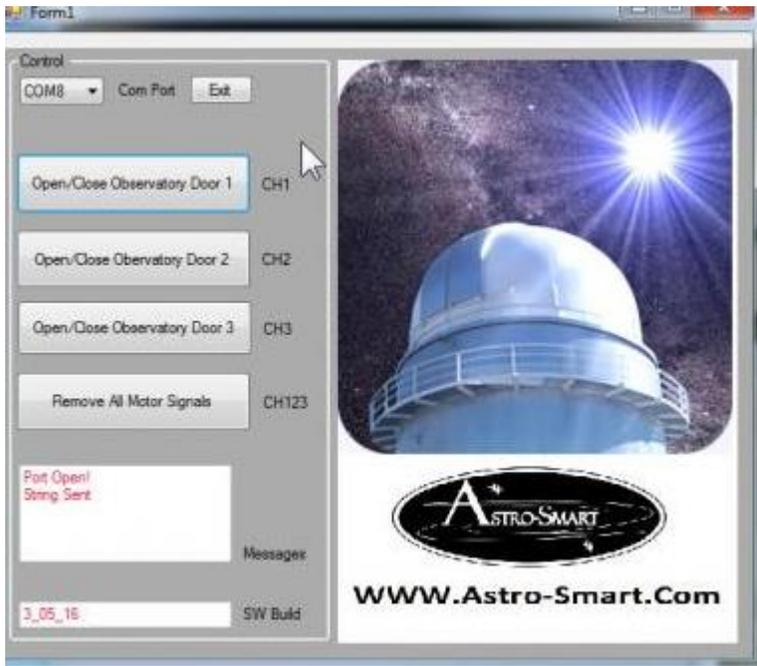
The PC SW remote interface snap shot main screen is shown to the left. Its a USB-Serial connection to the COSC Pro tested across multiple PC operating system platforms.
