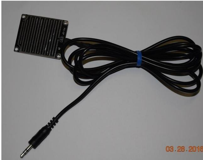
Optional accessory that Astro-Smart offers is the Rain Sensor used for automatic output channel control to shut observatory door when rain detected. Placement of sensor can be inside observatory when the door is open and sensor is exposed to night sky.
