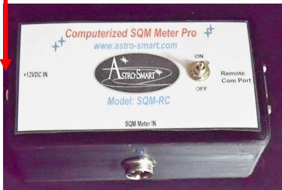
Figure 2 DC power plug
